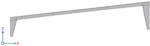
3 Clear Span, Single Slope Rigid Frame
